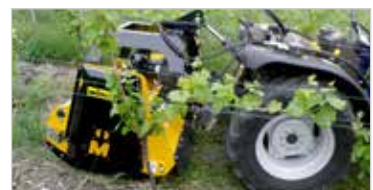
Gear box with twin freewheels enables use on tractors with different PTO shaft rotation directions (optional)
