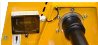
Operating hours counter with sensor, time recording using rotation pulse
