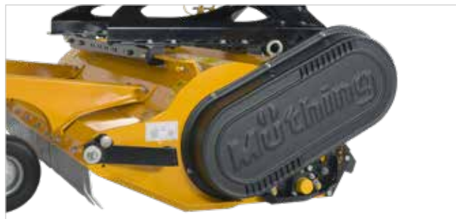
HDPE V-belt protective cover with inspection opening
