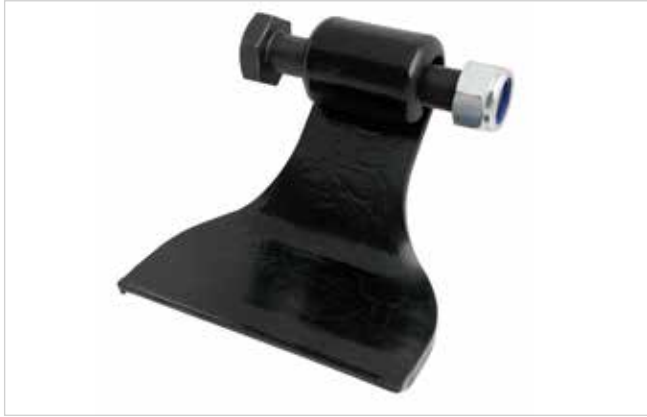
Rolled steel special MU-Farmer® hammer flail, 2.7 kg heavy with 3-year warranty against breakage, for shredding large quantities of organic matter
