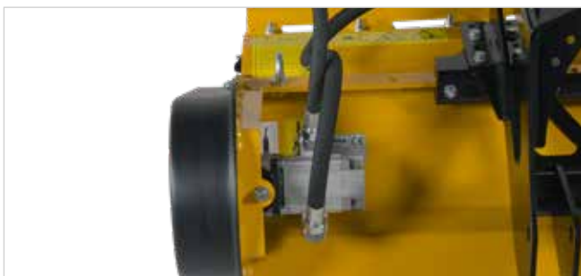
Sturdy, large and vertically adjustable support wheels, 360° swivelling (dia. approx. 235 mm and approx. 80 mm wide)
