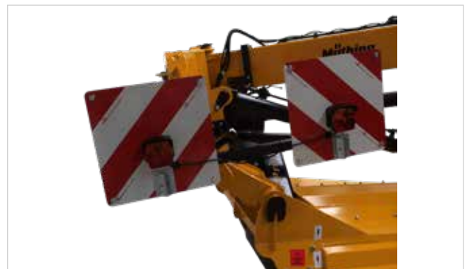
Warning signs with lighting equipment and lighting equipment support (fitted)
