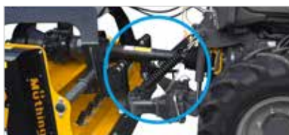
Improved steering capability and traction with front mounting thanks to the front shock-absorbing spring assembly (optional)
