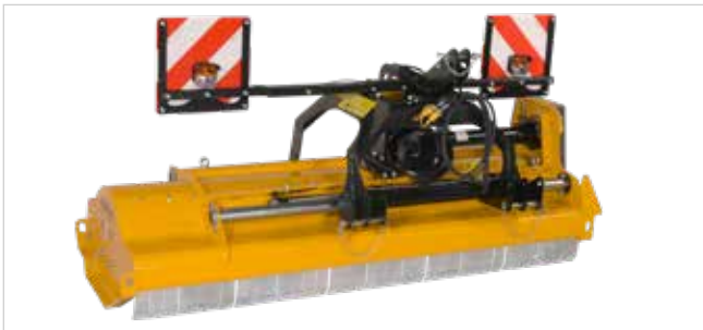
Special 3-point linkage Cat. 1 for carrier vehicles (e.g.: Aebi, Reform)
