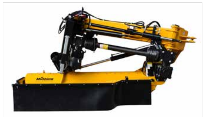
Additional protection device for extremely stony conditions as protection for tractors and carrier vehicles
