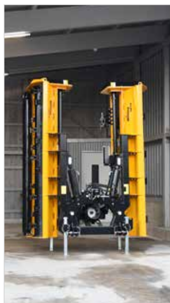
Hydraulically driven strip mulcher, for a perfect appearance and consistent results Required oil quantity: 50 l / 180 bar. Required hydraulic connections: 1 x pressure line with BG 2 plug 1 x pressureless return line with BG 3 socket, Max. back pressure < 20 bar
